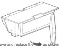
Remove and replace the filter as shown
