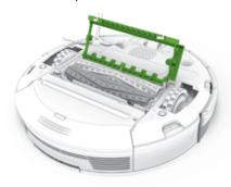
Remove the extractors and remove the yellow extractor caps. Remove any hair or debris that has collected underneath the caps and around the metal axles.
