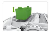
3 Reinstall the battery door and the two screws. Take care not to pinch the side brush in the battery door when re-installing the battery.
