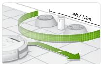
Virtual Wall Mode: When the switch is in the "up" position ( ••), the device functions as a Virtual Wall. This means that you can set it to block openings of up to 10 feet (3 meters). It creates an invisible, cone-shaped barrier that only Roomba can see.
