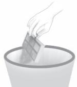
2 Shake off debris by tapping the filter against your trash container.
