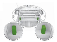
3 Wipe the inner and outer sensor ports on the bin with a clean, dry cloth.
