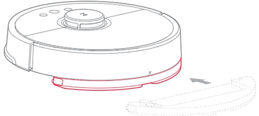
**Note:** In order to achieve a better mopping effect, it is recommended to use the main unit to clean the floor three times before install the mopping module.
