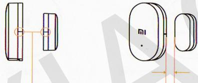
During installation, try as much as possible to balance the location of the primary sensor and the magnet at a special mark (see Figure 2)
