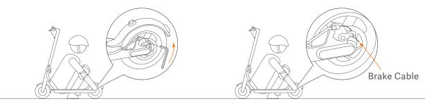
If the brake is too tight, use the 4 mm Allen key to loosen the screw on the caliper. Then slightly adjust the brake line (decrease the exposed length), and tighten the screw again. If the brake is too loose, loosen the screw on the caliper. Then slightly adjust the brake line (increase the exposed length), and tighten the screw again.
