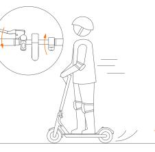
4. Release the accelerator and the kinetic energy recovery system (KERS) initiates automatically to brake slowly; squeeze the brake lever for a sudden brake.
