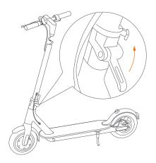
2. Install the handlebar onto the stem.
