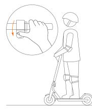
3. When the scooter starts to coast, put both feet on the deck and press the accelerator Note: The accelerator initiates once the coasting speed exceeds 5 km/h.
