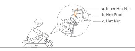
Long-term use of the scooter may result in loose screws, causing the handlebar stem to get unstable. If you notice the handlebar stem gets shaky when riding, follow the steps below.
