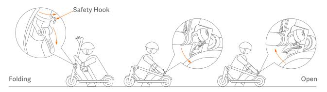
The scooter needs to be turned off before folding. Hold the handlebar stem, turn it counterclockwise to open the safety hook and open the quick release lever. Align the bell and the buckle and hook them.
