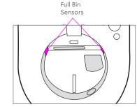
3 Remove the filter and wash the bin, or gently clean the bin to ensure the sensor ports are clean.
